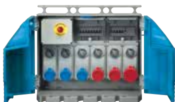
Assemblies for construction sites (ACS) with interlocked socket-outlets protected by MCB entry with inlet 50-60Hz IP65
