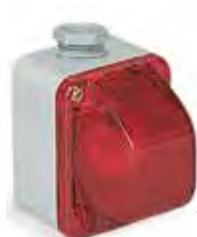
Signalling lamps in thermosetting GRP with E14 lamp holder for wall-mounting IP65
